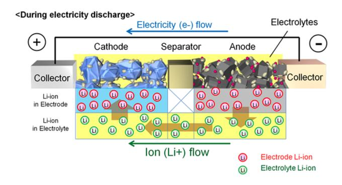
Structure and Principles of an Automotive Li-ion Battery
