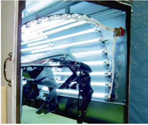
Next, Sakato and Chikao Kawamura, the Master Craftsman who specializes in paint application and finishing techniques, inspect the exterior under a range of different lighting conditions. Sakato uses a specially made light tunnel that allows him to examine the surface flow over the entire body and carefully compare it against the theoretical ideals of their CAD images. Kawamura goes over the paint job under three different simulated light conditions. Together, they
